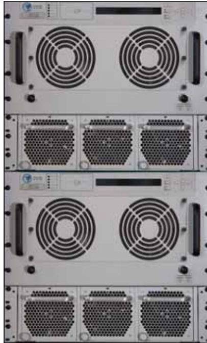
1.1 kW C-Band, 1:1 Redundant System in the 6RU Chassis
